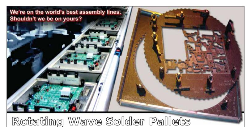
**Eliminate** bridges and skips, **reduce** rework and **increase** and **optimize** wave solder process reliability using Rotating Wave Solder Pallets from Pentagon EMS. Pentagon's Rotating Wave Solder Pallets allow you to **eliminate the guesswork** by **testing to determine the best angle** of PCB presentation to the wave **before** purchasing dedicated tooling.
